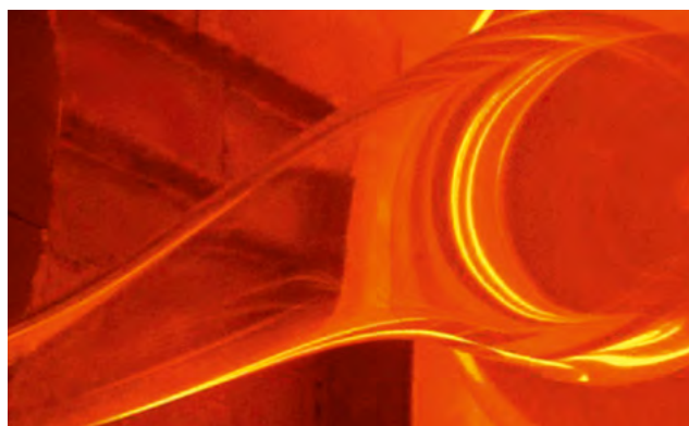
Tube forming with Danner-system
