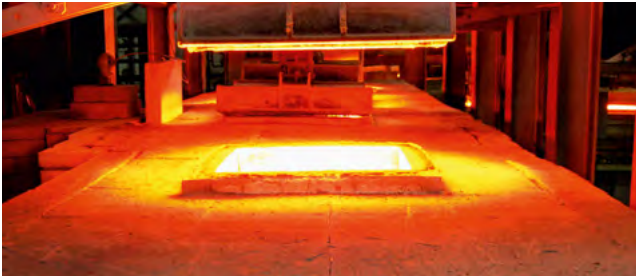
Distribution channel/forehearth superstructure insulation, with detail of flue openings
