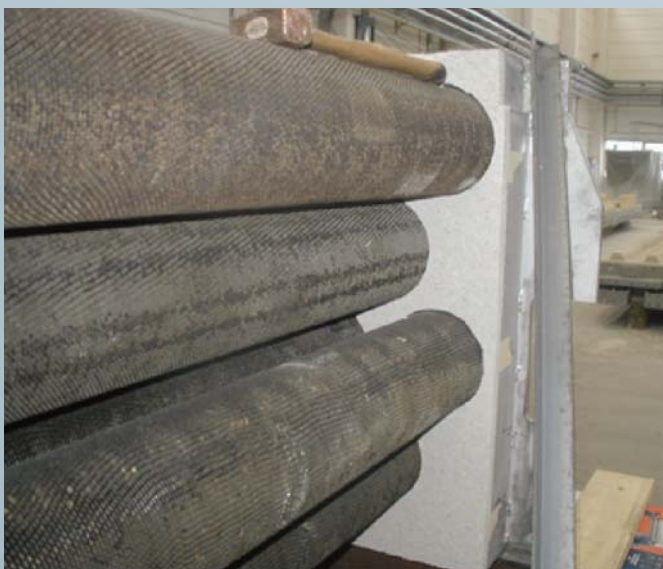
Convection zone tube shield (petrochemical cracker)
