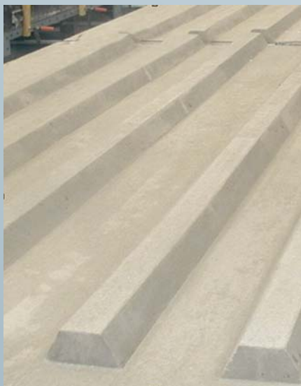
Convection zone panel (petrochemical cracker)
