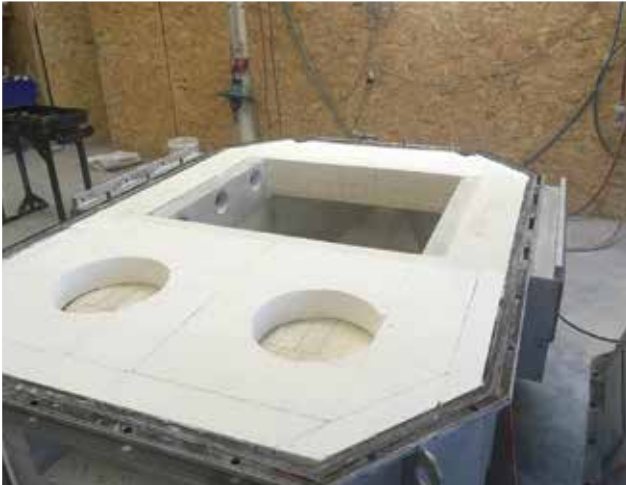
Dosing furnace–Top view
