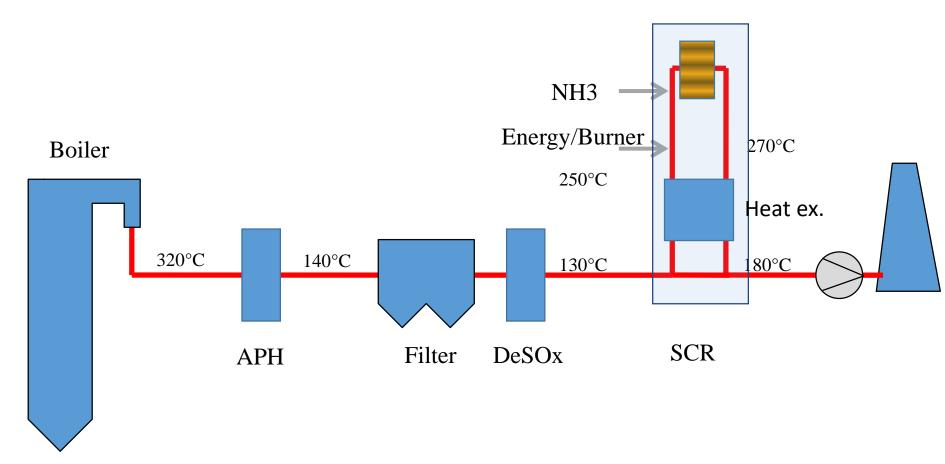
Low Dust SCR - Connected after dedusting, generally after DeSOx. Advantage: No dust, smaller catalyst volume, longer catalyst lifetime
