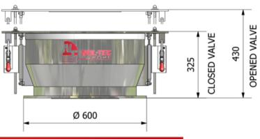
PNEUMATIC TENSIONING SYSTEM FOR DISCHARGE BULK BAG (OPTION)
